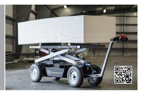
A rugged and self-propelled transport trolley with an electric lifter which raises up to 86 cm above ground level. The trolley has two side pockets for being lifted by a forklift.
